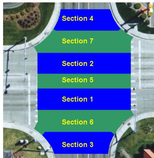
**Figure 4.** Concrete placement in interim Sections
