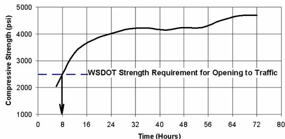
**Figure 2.** Compressive strength gain vs. time
