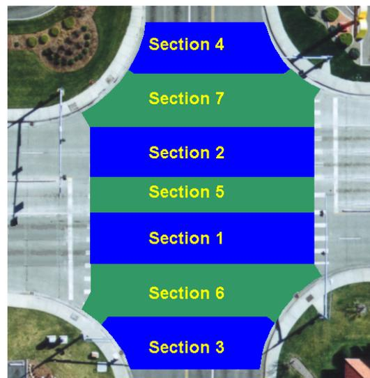
**Figure 4.** Concrete placement in interim Sections
