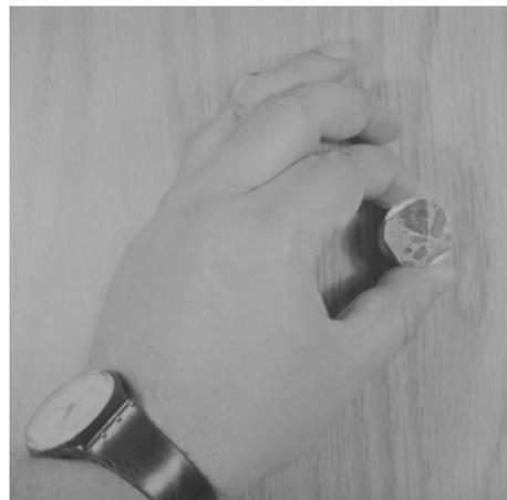
**Figure 2.24** Specimen placed on glass plate and aluminum base for SEM study
