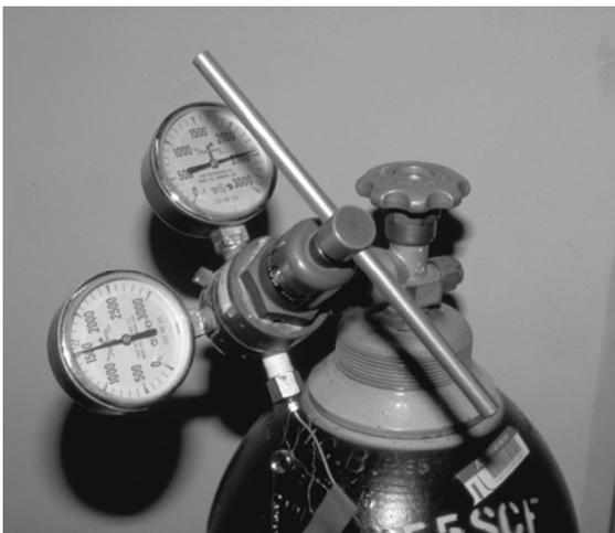
**Figure 2.14** Nitrogen dispensed through a high pressure regulator
