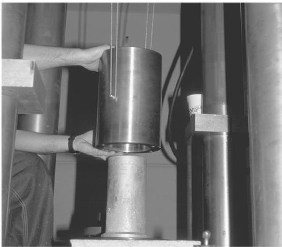
**Figure 2.18** Raising the vessel by aircraft cable
