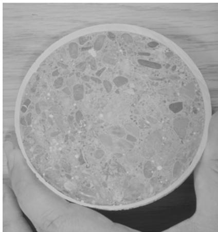
**Figure 2.23** A lateral section showing macrocracks filled with metal alloy
