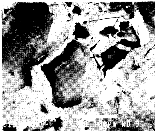
FIG. 11. Secondary Electron Image of Etched Sample Showing Grain Boundary Microcracks
