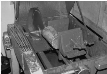
**Figure 2.20** Axial cut of concrete cylinder
