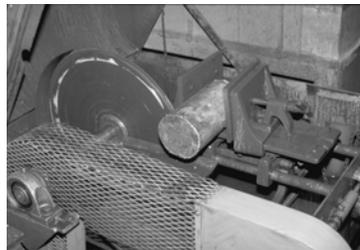
**Figure 2.21** Lateral cut of concrete cylinder
